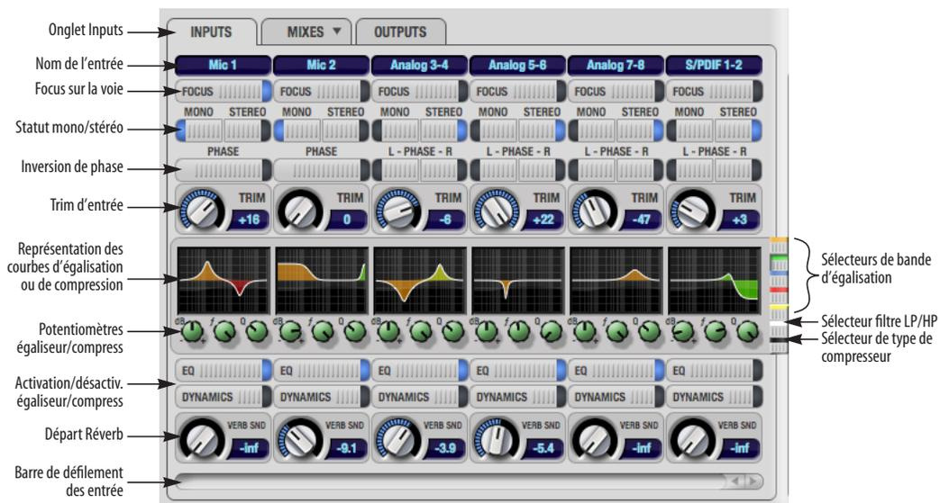
Figure 11-3 : L'onglet Inputs.
